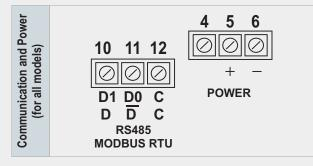
Obs.: Terminals 6 and 12 are connected internally.
