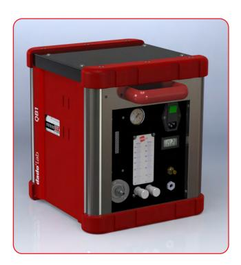
Each QB1 sampler manufactured is thoroughly tested and its calibration verified through certified references traceable to international standards.
