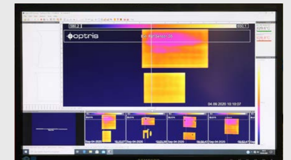
Monitoring temperatures of glass sheets
